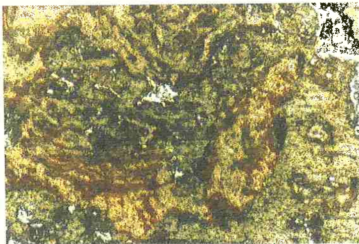
Figura 16: Microscopia Óptica - 100x - FeO+Silica
