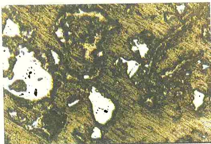
Figura 18: Microscopia Óptica - 100x - FeO+Silica
